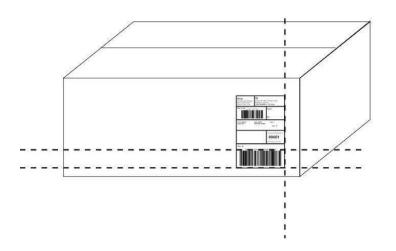
No matter the carton height, always place your GS1-128 label in the bottom right hand corner of the carton of the longest side. If a shorter carton, you may fold over the upper portion of the GS1-128 label.
